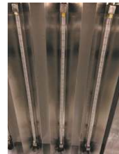
Curing zone with heating tube and reflector
