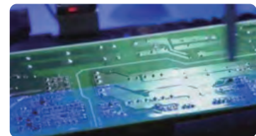
Thin film valve achieving clear spraying boundary
