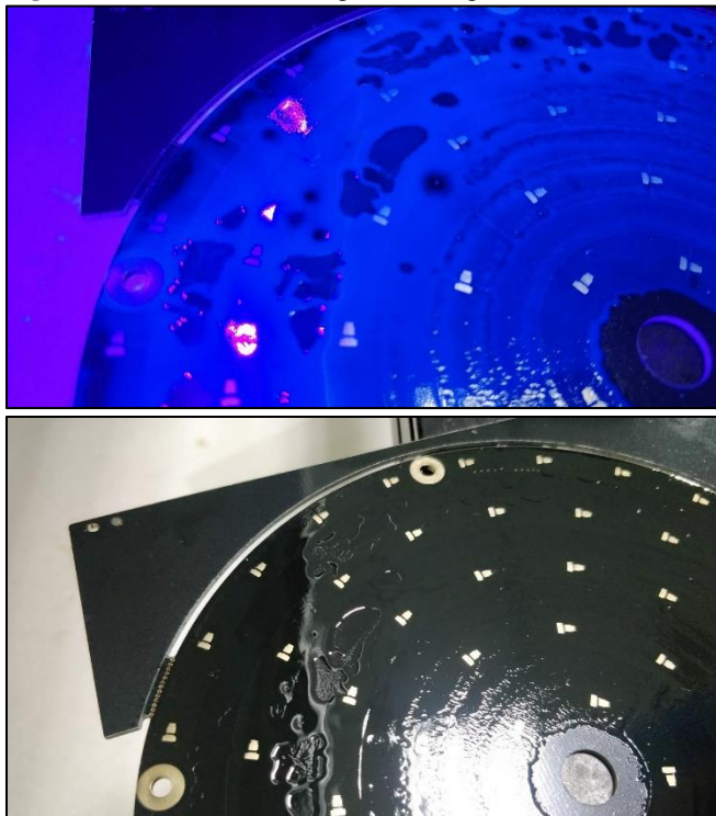
Figure 1: Conformal Coating Dewetting
