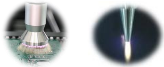
Figure 8: 50mm Rotation Nozzle (left) and 6mm Spear Nozzle (right)
